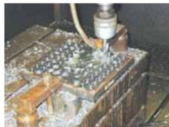
As ABREX steel plate is extremely hard and this can make it difficult to form and process, we recommend any drilling take place in a machining center using an ultra-hard metal alloy drill. However, for smaller jobs and working with components, it is often the case that boor-bank drilling machines and high-speed steel drills are used, so here we will introduce our recommended approach to drilling ABREX steel plate using a high-speed steel drill.
